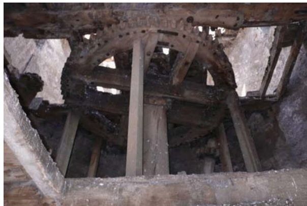
Plate 12 Upright shaft and great spur wheel
